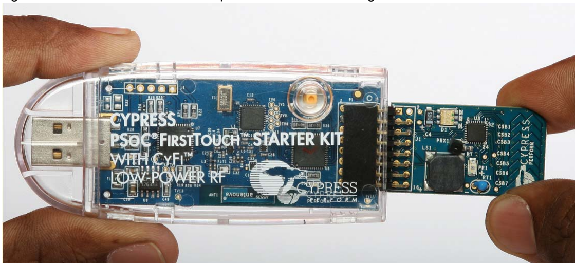
Figure 3-8. Connect Multifunction Expansion Card to PC Bridge
