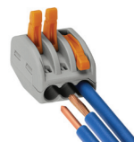
222-413 3-Pole Cage Clamp Conductor sizes: 0.08mm 2 - 2.5mm 2 Solid Core 0.08mm 2 - 4.0mm 2 Stranded Core Current rating: 32A Voltage rating: 400V/4KV
