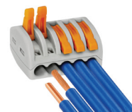
222-415 5-Pole Cage Clamp Conductor sizes: 0.08mm 2 - 2.5mm 2 Solid Core 0.08mm 2 - 4.0mm 2 Stranded Core Current rating: 32A Voltage rating: 400V/4KV
