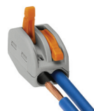
222-412 2-Pole Cage Clamp Conductor sizes: 0.08mm 2 - 2.5mm 2 Solid Core 0.08mm 2 - 4.0mm 2 Stranded Core Current rating: 32A Voltage rating: 400V/4KV
