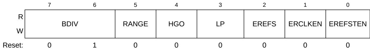
Figure 8-4. MCG Control Register 2 (MCGC2)
