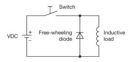
Counter EMF over load without free-wheeling diode Fig. 2
