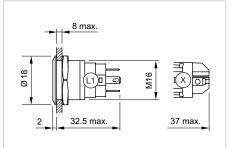
Dimensions [mm]  $L1 = Solder/Plug-in terminal 2.8 \times 0.5 mm, X = Screw terminal$
