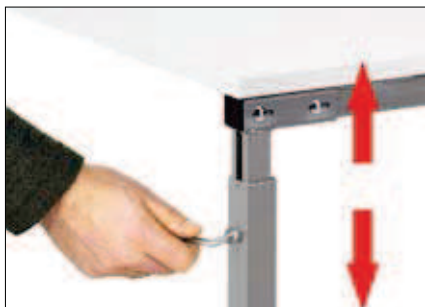
Stepless height adjustment with allen-key between 650...900 mm
