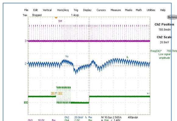
Figure 45: External frequency synchronization to 800KHz from free running 600KHz, Ch2:Vo, Ch3:LX, Ch4:Rt/Sync Voltage
