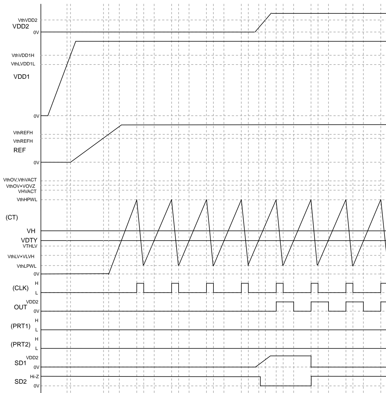
Figure 4. VDD1 Start to VDD2 Start Timing Chart
