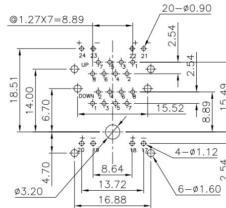
PC Board Layout Thickness=1.6mm
