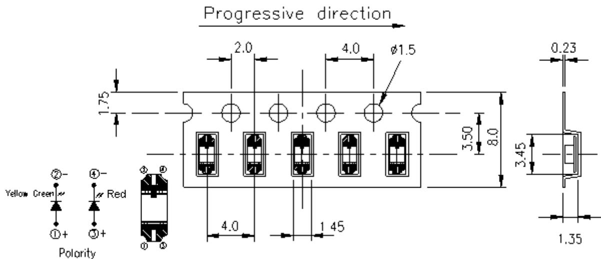
**Note:** The tolerances unless mentioned is  $\pm 0.1\text{mm}$ , Unit = mm
