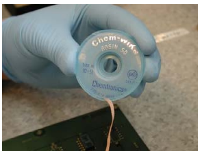
Figure 15. Soldering iron and solder braid used for solder removal.
