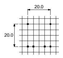
PCB Pins 0.635mm Sq Pin length 5.0mm Hole size 1.0mm
