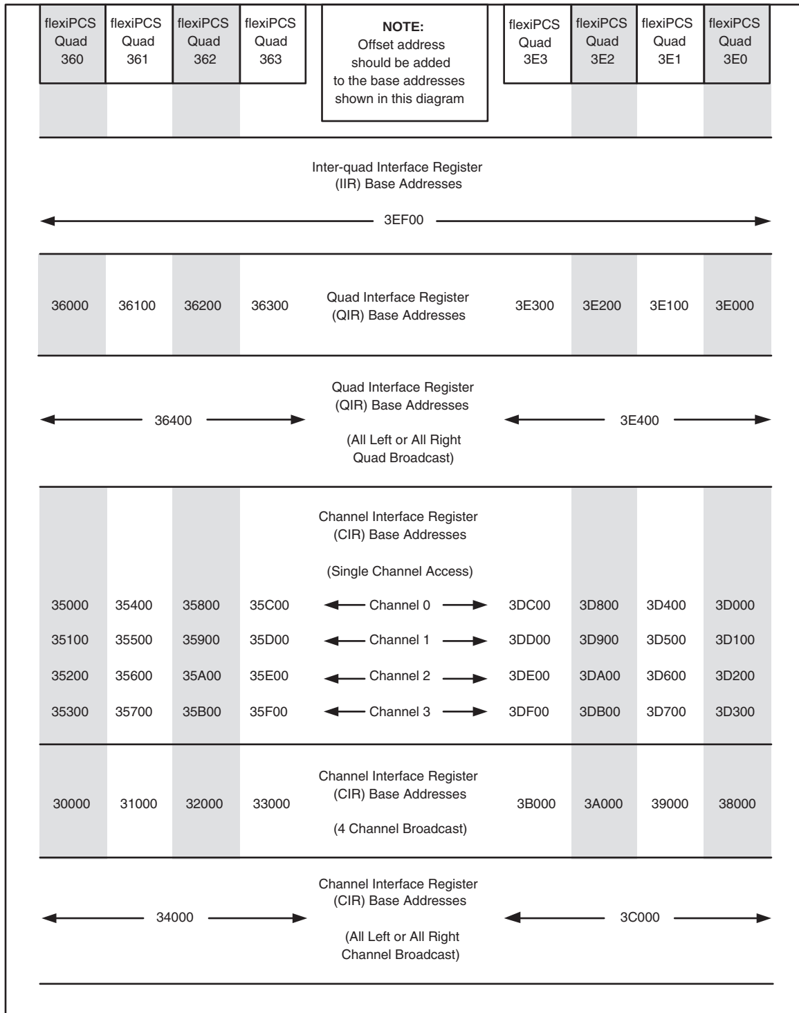
Figure 3-1. flexiPCS Inter-quad, Quad, and Channel Interface Register Map Base Addressing
