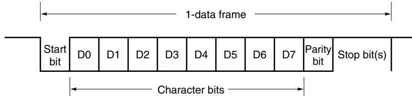
Figure 16-7. Format of Asynchronous Serial Interface Transmit/Receive Data
