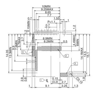
Note 1 > 4 indicates the center line of the microSD card slot.
