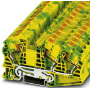
Ground modular terminal block, Connection method: Push-in connection, Cross section: 0.5 mm 2 - 25 mm 2 , AWG: 20 - 4, Width: 12.2 mm, Color: green-yellow, Mounting type: NS 35/7,5, NS 35/15
