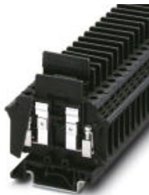
Fuse terminal block for cartridge fuse inserts 5 x 20 and 5 x 25, cross section: 0.2 - 4 mm 2 , width: 8.2 mm, color: blue
