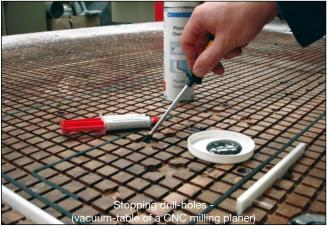
WEICON Epoxy Minute Adhesive and WEICON Fast-Metal Minute Adhesive are especially suitable for occasionally necessary repair and maintenance works. They are applied by using the practical double syringe. This means that resin and hardener are delivered automatically in the right proportions. After this, the mixing is done manually.
