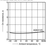
2.-(2) On resistance vs. ambient temperature characteristics
