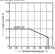
1.-(2) Load current vs. ambient temperature characteristics
