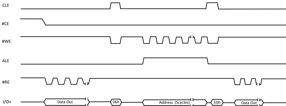
Figure 9-4 Two Plane Random Data Read (06h-E0h) Operation
