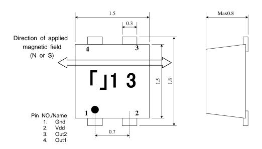
Coplanarity: less than 0.1mm(includiong under reflow condition)
