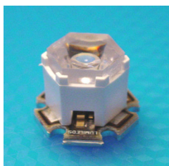
121 Holder and 120 Optic mounted on LUXEON® I Star PCB
