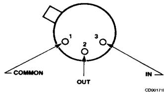
Lead 3 connected to case.
