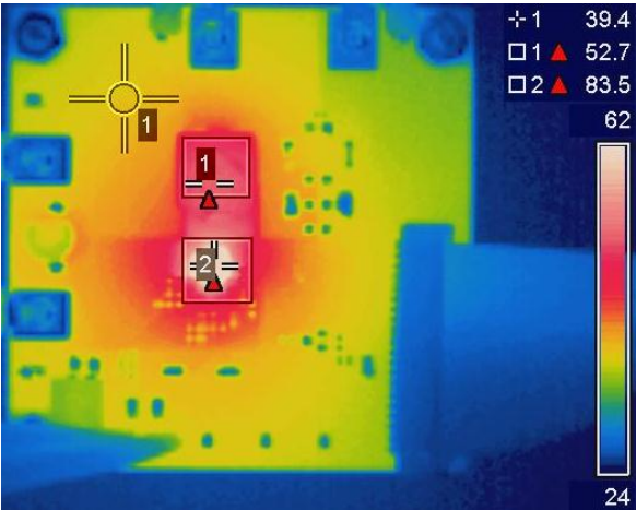
Figure 19: Thermal Image at VIN = 16V, IOUT = 10A (IR3865: 84°C, Inductor: 53°C, PCB: 39°C)
