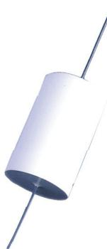
Type 935 metallized polypropylene capacitors are designed for filtering applications in switching power supplies that operate in the 20-100 kHz range. Their low ESR, high current and high capacitance gives them an advantage over general purpose types. This series is UL recognized for construction only under UL File Number E128034(N).
