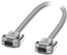
Assembled shielded round cable; Connection 1: D-SUB socket strip (1x 9-position); Connection 2: D-SUB pin strip (1x 9-position); Cable length: 2 m
