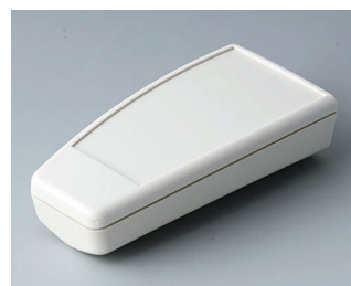
A9066317 SMART-CASE M, Vers. VI ABS (UL 94 HB) off-white RAL 9002 3.78"x1.85"x0.94" IP 40
