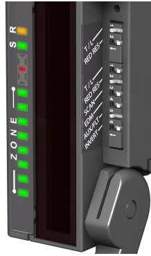
Figure 55. DIP switch configuration to enable cascade installation
