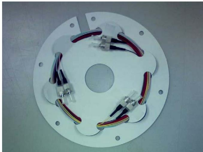
These coloured pigtails complement the use of colour coded fibre in loose tube cables. Usually 12 different colours are used in either IEC or Bellcore coding. These pigtails use the same 12 colours, thus can be used for applications with both colour codes. The use of these colour coded pigtails makes the termination of fibre cable in patch panels or termination terminals easier and safer. Due to clear dedications, the risk of wrong fibre connections is reduced.
