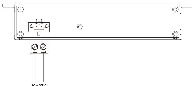
Figure 2-20 Power Connection for EDG-4504
