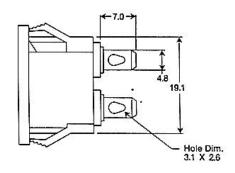
Universal snap-in tabs allow for insertion into a wide variety of panel thicknesses. Conforms with all international safety requirements. Rated 15 Amp., 250 VAC for ?? and ?? 10 Amp., 250 VAC for ?? 65°C operating temperature.
