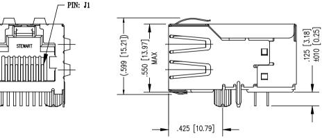
1. CONNECTOR MATERIALS: HOUSING: THERMOPLASTIC UL94 V-0
