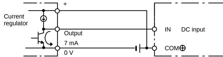
NPN open-collector output
