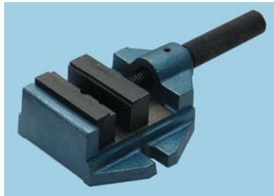
Small drill vice for use in drilling and light milling operations. Effectively grips round, square, thin and irregular sections. The jaws are made of hardened steel and base cast iron. Handle is mounted on ball bearings to give more gripping power, smooth action and long life.
