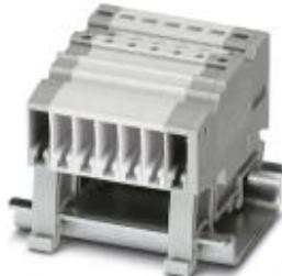
COMBI receptacle, Connection method: Push-in connection, Number of positions: 14, Cross section: 0.14 mm<sup>2</sup> - 1.5 mm<sup>2</sup>, AWG: 26 - 14, Width: 49 mm, Height: 27.1 mm, Color: green/yellow-gray, Mounting type: NS 35/15, NS 35/7,5
