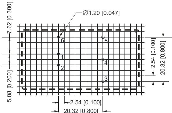
Pin section tolerances: ±0.10 mm [±0.004 inch]
