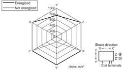
Measurement conditions: Impose a shock in the  $\pm X$ ,  $\pm Y$ , and ±Z directions three times each with the Relay energized to check the shock values that cause the Relay to malfunction.
