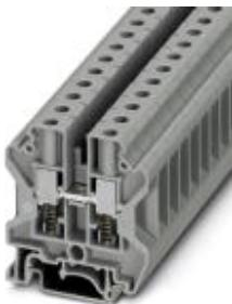
Feed-through terminal block, Connection method: Screw connection with spring support, Cross section: 0.5 mm<sup>2</sup> - 16 mm<sup>2</sup>, AWG: 20 - 6, Width: 10.2 mm, Color: gray, Mounting type: NS 35/7,5, NS 35/15, NS 32
