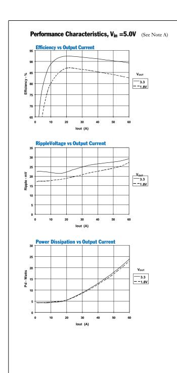
Note A: Characteristic data has been developed from actual products tested at 25°C. This data is considered typical for the regulator.
