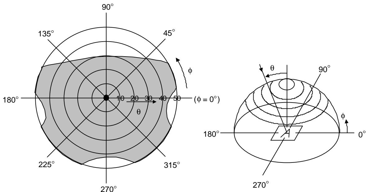
\*Area shows typ.  $CR \geq 2$  (Measuring Spot : 3.0mmφ)
