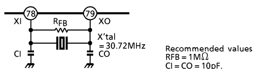
Fig.1(a) Self excited crystal oscillator
