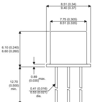
**Bipolar NPN Device in a
