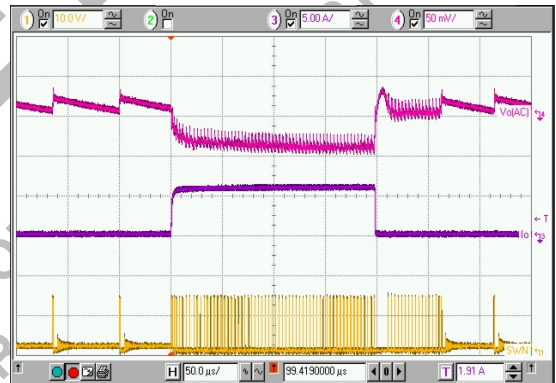
Top: Vo2, CH2 Output Voltage Ripple, (50mV/div) Middle: Io2, CH2 Output Current, (5A/div) Bottom: SWN2, CH2 Switching Node Voltage, (10V/div) Time: 50μs/div
