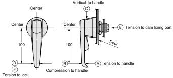
Applied Force Directions of Tension, Compression, Vertical, and Torsion
