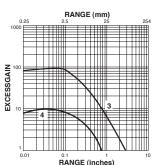
Gain using E51KF723 fibers, based on 90% reflective white card
