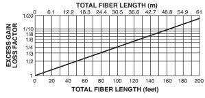
② Sensing range is based on 6 ft (2m) of plastic 1 mm diameter source and detector fiber optic cable for a total length of 13.1 ft (4m). To determine performance with longer lengths, see graph above.
