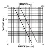
Gain using E51KF823 fibers
