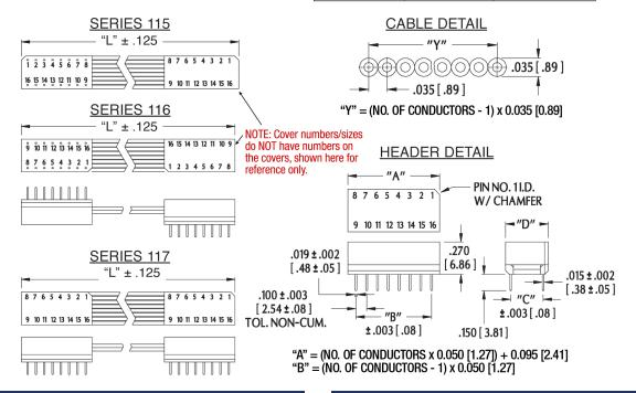
**ALL DIMENSIONS: INCHES [MILLIMETERS]** ALL TOLERANCES: ±0.005 [0.13] UNLESS OTHERWISE SPECIFIED CONSULT FACTORY FOR OTHER SIZES AND CONFIGURATIONS
