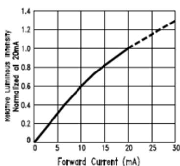
Fig.4 Relative Luminous Intensity
