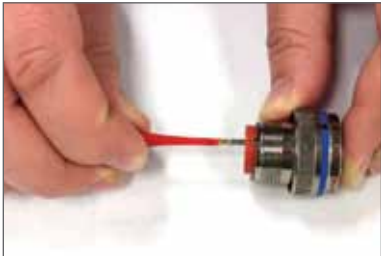
Plastic tool with contact in proper position.
