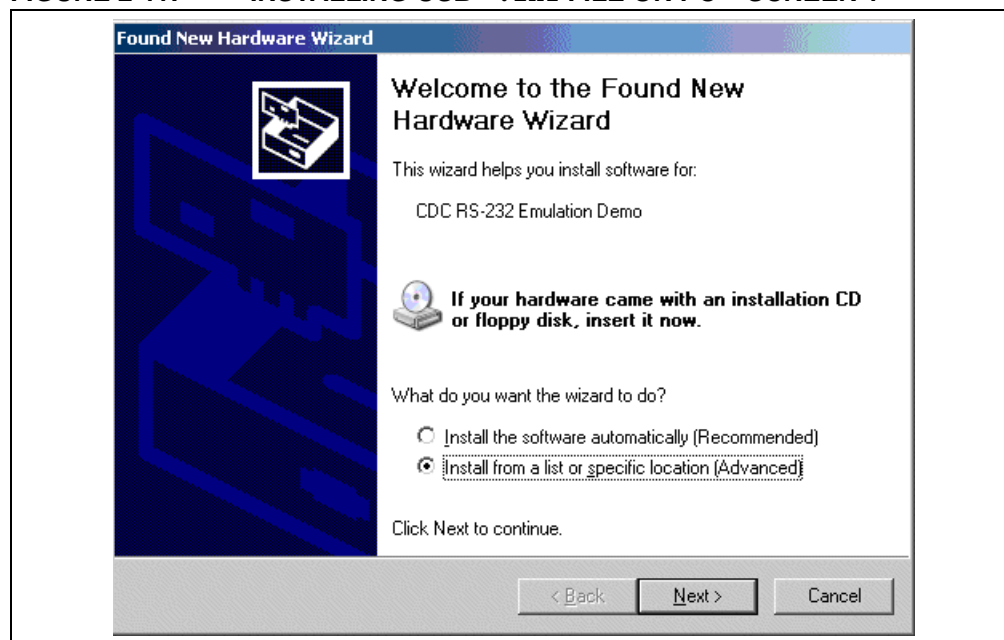
FIGURE 2-11: INSTALLING USB *.inf FILE ON PC – SCREEN 1
