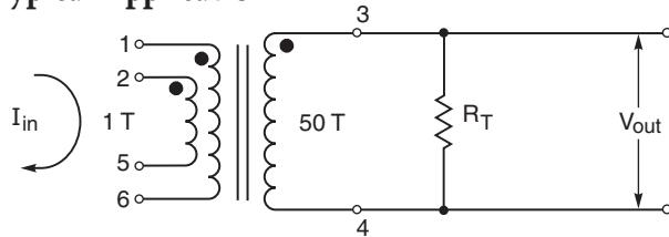
Varying the terminating resistance ( $R_T$ ) increases or decreases output voltage/Ampere in conductor.
