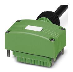
Connector hood, Number of slots: 8, Slot assignment: Double, Status indication: No; Master cable connection: Pluggable screw connection 180°, PUR/PVC, Cable length: 25 m, Shielding: No
